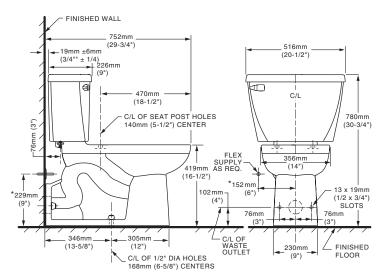
WASTE OUTLET SEAL RING MUST BE NEOPRENE OR GRAPHITE-FELT (WAX RING NOT RECOMMENDED).
