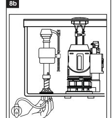
With correct washers in place (see Step 8a), tighten COUPLING NUT 1/4 turn beyond hand tight.
