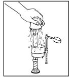
IMPORTANT: Always clear sand and rust from system. • Make sure water supply is off. Remove valve TOP by lifting arm and rotating top and arm 1/8 turn counterclockwise, pressing
