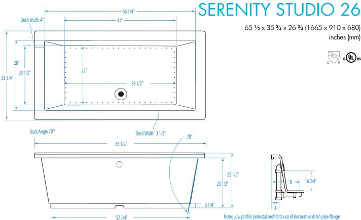
FEATURES | lbs (kg) | Dimensional Tolerance ± 3/8". Dimensions needed for site preparation should be measured from the unit. Aquatic assumes no responsibility for preparatory work.
