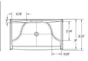
FEATURES | Ibs (kg) Dimensional Tolerance ± %". Dimensions needed for site preparation should be measured from the unit. Aquatic assumes no responsibility for preparatory work.
