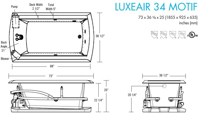
FEATURES Ibs (kg) Dimensional Tolerance ± 3/8". Dimensions needed for site preparation should be measured from the unit. Aquatic assumes no responsibility for preparatory work.
