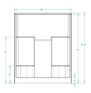
AFR: Allows for above the floor installation of waste, overflow and drainage.
