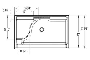
FEATURES | Ibs (kg) Dimensional Tolerance ± %". Dimensions needed for site preparation should be measured from the unit. Aquatic assumes no responsibility for preparatory work.
