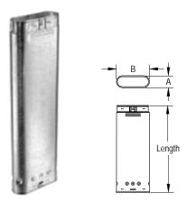
Use for venting listed natural gas or liquid propane Category I, draft hood appliances, or appliances that have been specifically tested and listed to use Type B Gas Vent. The appliances listed typically use Type B Gas Vent systems, but not always: Furnaces, Water Heaters, Boilers, Room Heaters, Decorative Gas Appliances, and Unit Heaters. Designed to be placed within 2" x 4" stud walls (4" and 5" oval pipe). 6" may only be placed in a 2" x 6" 16" O.C. stud space.
