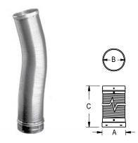
Round-to-Round Flex pipe built from .016", 304 stainless steel, 4-ply construction. Use through damper and smoke shelf area. Features built-in fittings, which eliminates field cutting and fitting. Use with DuraLiner Two-Ply Insulation Sleeve for zero clearance applications where flex extends into clay liner.
