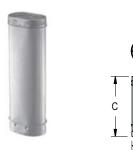
Factory insulated, Oval Rigid Pipe is available in 6" and 8" diameters; 12", 24", 36", and 48" lengths. Insulated. Built-in pre drilled fittings for riveting joints. UL Listed for zero clearance between masonry and combustibles, plus zero clearance between liner and masonry. 304 stainless steel inner and aluminized steel outer.
