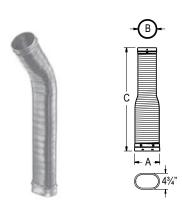
Use through damper and smoke shelf area. Use to connect from oval stove outlet to round DuraLiner. Built from 304 stainless steel. Use with DuraLiner Two-Ply insulation Sleeve for zero clearance applications where flex extends into clay liner.
