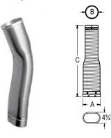
Oval-to-Round flex pipe built from .016", 304 stainless steel, 4-ply construction. Use through damper and smoke shelf area. Use to connect from oval stove outlet to round DuraLiner. Use with DuraLiner Two-Ply insulation Sleeve for zero clearance applications where flex extends into clay liner.
