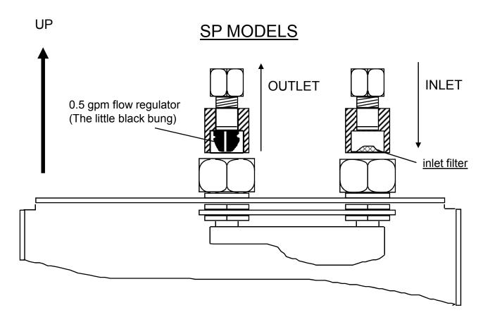
If the heater now turns "on" with water flowing, call Eemax at 1-800-543-6163. Describe what you have done and we will send you a selection of "bungs" to replace the one which you have removed. This will allow the unit to turn "on" but will also control the flow rate to give you the correct rise in temperature.
