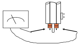
If the reading is less than 20 ohms on the "Rx 1" scale or the "Rx 10" scale the element is good, if it is much greater e.g.... 10,000 ohms or if you get a reading on the "Rx 1K" scale then you must replace the element (contact Eemax). Tel : 1-800-543-6163 for replacement elements.
