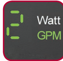
Large display shows estimated flow in gallons per minute
