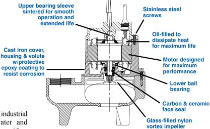
For residential, medium commercial and light industrial applications, the Model 9S Series Wastewater and Sewage Ejector pumps feature a 2" discharge, with a maximum lift of 18'. Cast iron housing, cover and volute have a protective epoxy coating.
