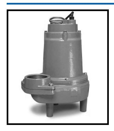
For residential, commercial, industrial and agricultural use. The model 14S Series Wastewater and Sewage Ejector pumps handle liquids and solid waste materials up to 2" in diameter. Pumps feature either a 2" or 3" FNPT discharge with a maximum head of 25', heavy duty cast iron construction and stainless steel hardware.
