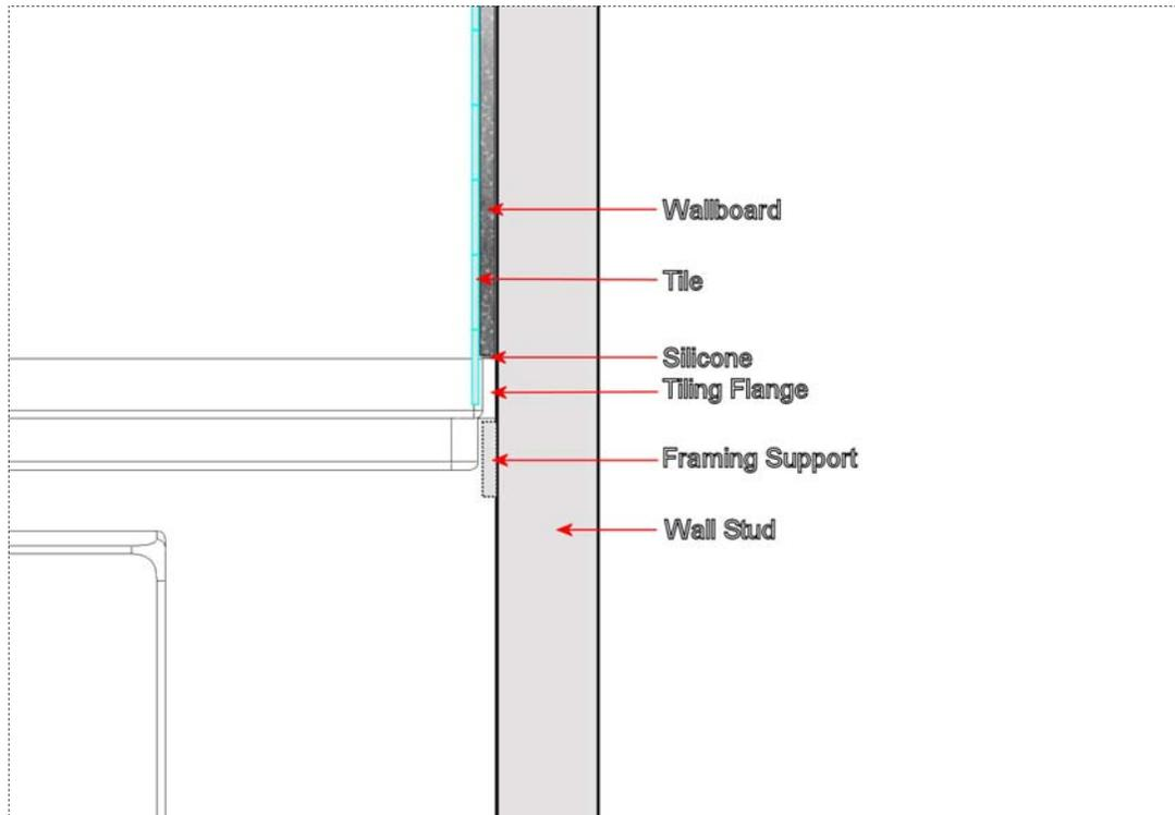
Typical Installation of Wallboarding And Tile - Section View
