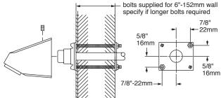
Anchor plate used for ceramic tile application—plate screws to wall and tile is applied up to sides of plate. Mounting bracket is mounted on finished wall with machine screws into anchor plate
