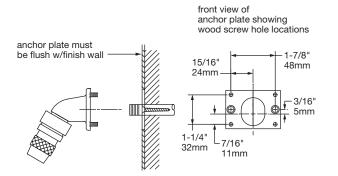
Anchor plate used for ceramic tile application—plate screws to wall and tile is applied up to sides of plate. Mounting bracket is mounted on finished wall with machine screws into anchor plate
