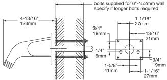
Anchor plate used for ceramic tile application—plate screws to wall and tile is applied up to sides of plate. Mounting bracket is mounted on finished wall with machine screws into anchor plate
