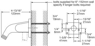
Anchor plate used for ceramic tile application—plate screws to wall and tile is applied up to sides of plate. Mounting bracket is mounted on finished wall with machine screws into anchor plate
