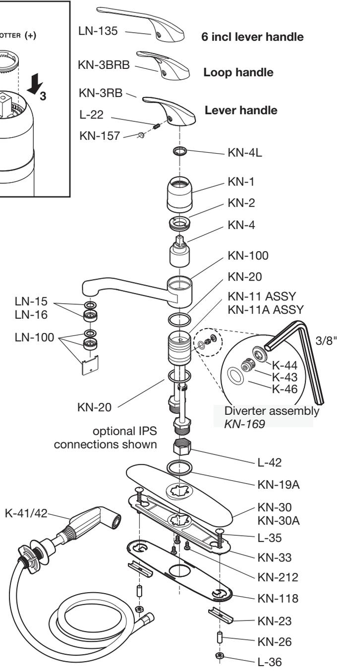
\* Note: When ordering parts for products with an optional decorative finish, append appropriate three letter finish suffix code to part numbers marked with an asterisk (\*).
