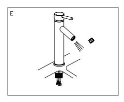
E. Turn on water supply to check for leaks at all connection. Remove aerator from the spout and let thewater run for about 1 minute and check for leaks. Reattach the Areator.
