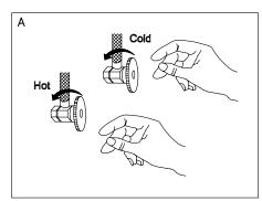
A. Shut off water supply at the valves. Remove old faucet and clean the mounting surface for instllation of new faucet.
