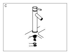
C. From under the sink, install the meatl wahser (14)and nuts (15) onto the mounting tube (13) Tighten the nuts to secure the faucet to the mounting surface.
