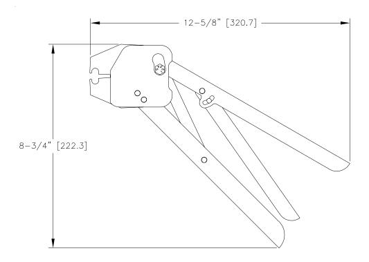
**Engineering Specification:** Zurn QickClamp™ Crimp Ring Tool. The QCRTQCM is a calibrated tool that applies the recommended force needed to make a leak-free crimp connection. The crimp tool is used with the QickClamp™ crimp rings, the Qick/Sert1® or QickSert CR™ fittings, and ZurnPEX® tubing to make a leak-free plumbing system.
