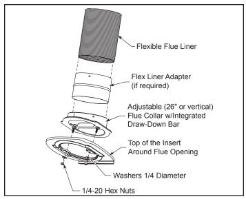
Figure 6 - Components of the venting system.
