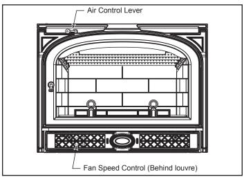
Figure 8 - Montpelier Medium Insert controls.
