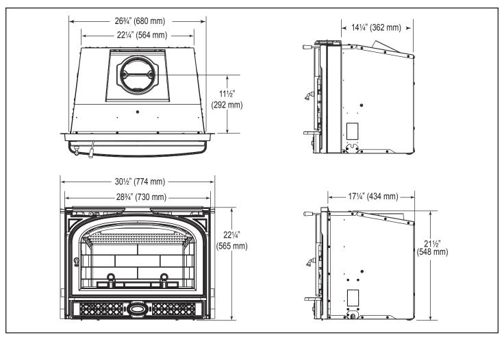
Figure 1 - Montpelier Medium Insert dimensions.
