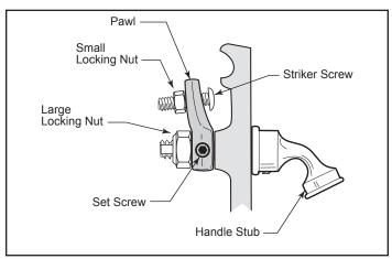
**Figure 12** - Turn the door latch striker screw in or out to tighten or loosen the door latch.
