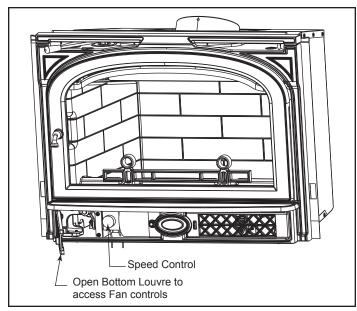
Figure 10 - Fan control access.
