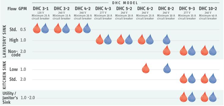
DHC 3-1, 3-2, 4-2 ship with a 0.5 GPM pressure compensating flow reducer/aerator that must be installed.
