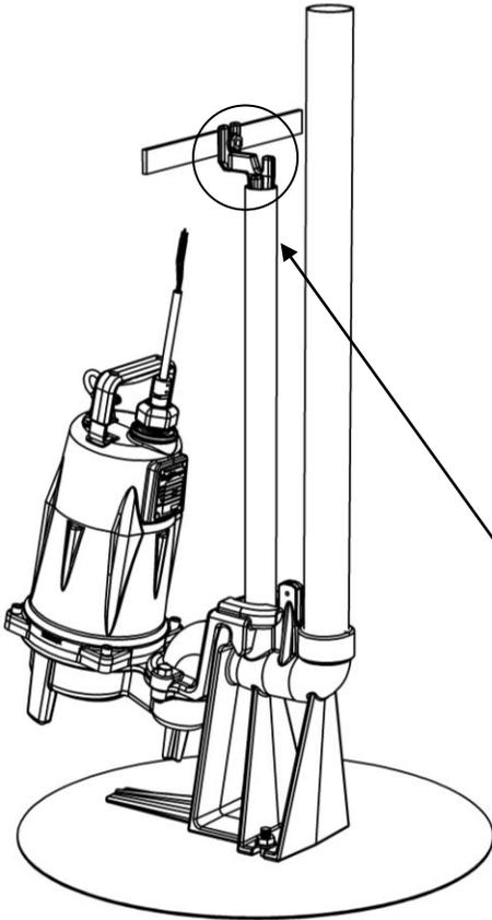
All the claws have a sealing grommet attached to it that provides the seal between the claw and base unit. This seal requires no maintenance. On GR30, GR22-LE, AND GR22-FL a gasket should be used between the claw and pump – **the gasket and mounting hardware are provided with the pump.** The stock flange that is shipped with the pump should be removed and replaced with the claw.
