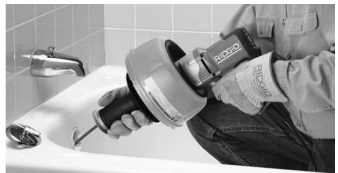
Figure 9 – Push Cable Down Drain Line
