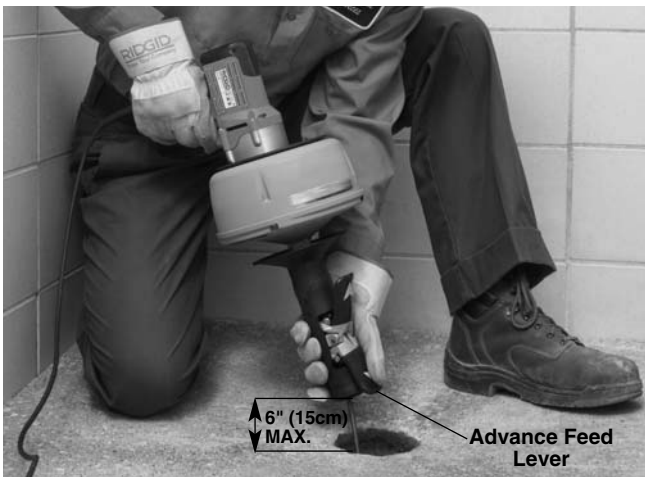
Figure 10 – Feeding Cable With AUTOFEED
