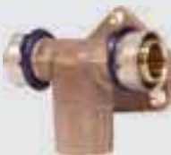
Viega PEX Press tee Zero Lead - For fire sprinkler systems - Bronze - Press connection, female pipe thread - Mounts to vertical surfaces Note For use with black ViegaPEX Ultra only. UL listed for NFPA 13D systems Model 2818.3ZL
