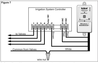
C. Controllers with pump start or master valve and no sensor inputs: Refer to Figure 8. Disconnect all common control wires from the common terminal(s) of the controller (generally marked "C", "Com", or "VC"). Join these wires to the White wire using a wire nut. (Be sure to include the common wire from the Pump Start Relay in this connection). Attach the Brown wire to the common terminal.
