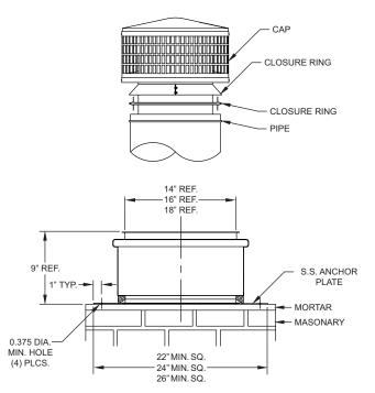
FIG. 15b 14TG, 16TG, AND 18TG ANCHOR PLATE
