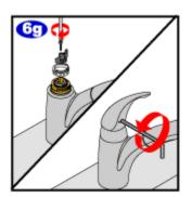
Reinsert your white pivot stop, secure the handle adapter to the cartridge stem, screw on your black plastic pivot retainer and replace the decorative dome. Lastly, reattach the handle. Go to step 8 if you want to reverse the Hot and Cold sides.
