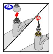
Lift off the decorative dome, unscrew the black plastic pivot retainer, and remove it. Remove the connector screw and lift off the adaptor and connector assembly. Next, remove the white handle stop.
