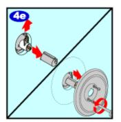
To reinstall the cartridge into your faucet assembly, reverse the steps that you followed to remove the old cartridge. Reinstall the retaining clip, the limit stop and the washer onto the cartridge. Fasten the escutcheon to the wall.
