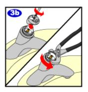
Unscrew the Philips screw and remove the adapter.
