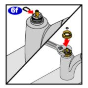
To reinstall the cartridge into your faucet assembly, reverse the steps that you followed to remove the old cartridge. Reinstall the washer onto the cartridge stem and reattach the retainer nut with adjustable pliers.
