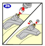
Pull the handle off from the faucet and pull the limit stop off. Remove the washer from the cartridge and use pliers to remove the retaining clip. Pull the stemp up on the old cartridge to relieve any pressure in the faucet.
