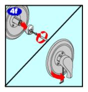
Replace the handle adapter, and finally secure the handle using the hex key. Go to step 8 if you want to reverse the Hot and Cold sides.
