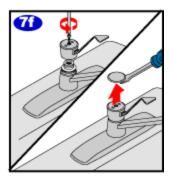
To reattach the handle, align the flat edge of the metal lever under the ridge on the retainer nut, towards the back of the nut. Then bring the handle down in the front so it drops into place. Secure the handle with the screw and snap the handle cover into place. Go to step 8 if you want to reverse the Hot and Cold sides.
