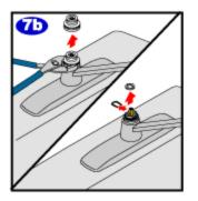
Using pliers, loosen and remove the pivot retainer nut as well. Remove the washer from the cartridge. Pull the stem up on the old cartridge to relieve any pressure in the faucet then use pliers to remove the retaining clip.
