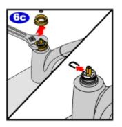
Unscrew the retainer nut using a crescent wrench. Pull off the washer from the cartridge and use pliers to remove the retaining clip.
