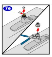
To reinstall the cartridge into your faucet assembly, reverse the steps that you followed to remove the old cartridge. Replace the washer onto the cartridge stem. Using pliers, secure the pivot retainer nut to the faucet assembly.
