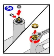
To reinstall the cartridge into your faucet assembly, reverse the steps that you followed to remove the old cartridge. Reinstall the washer onto the cartridge stem and reattach the retainer nut.
