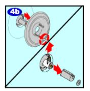
To get access to the cartridge, unscrew and remove the faucet escutcheon. Remove the washer and the limit stop from the cartridge and use pliers to remove the retaining clip.
