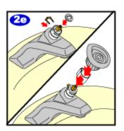
Reinstall the clip and replace the washer onto the cartridge. Then replace the stop tube, and replace and secure the handle. Finally, snap the handle cover into place. Go to step 8 if you want to reverse the Hot and Cold sides.
