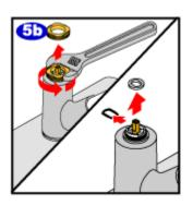
Using an adjustable wrench or a pair of adjustable pliers, twist off the retainer nut. Pull off the washer from the cartridge.
