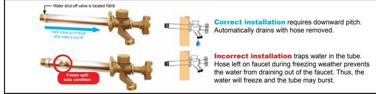
The faucet above is shown with the valve in the closed position. The water is shut off several inches into the home. The water line does not freeze because of the heat in the home. The product cannot freeze because there is no water in the faucet. When the valve is turned off, all of the water in front of the valve drains from the faucet leaving the tube empty. Also shown is correct and incorrect installation and a frozen split tube condition when hose is left on during freezing weather.
