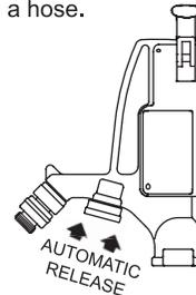
When the hydrant is closed to an OFF position, the diverter will automatically release, allowing the hydrant to drain into the reservoir. The hydrant will drain even if a pressurized or non pressurized hose is attached.
