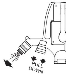
By pulling down on the diverter sleeve during flow, water will be diverted through the backflow preventer (BFP), and allow use with a hose.
