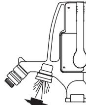
When the hydrant is opened to an ON position, water will flow through the diverter spout.
