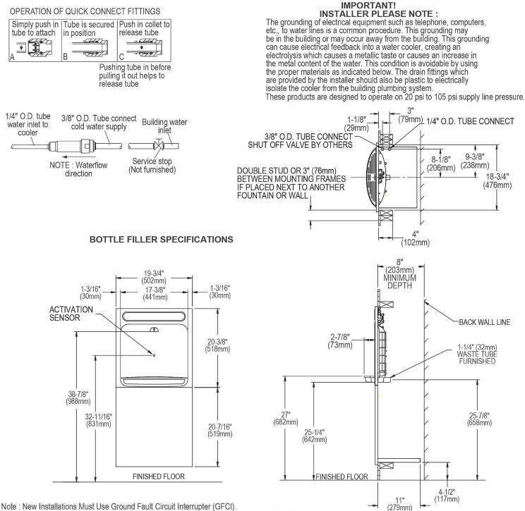
It is highly recommended that the circuit be dedicated and the load protection be sized for 20 amps.
