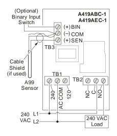
Figure 11: Wiring the 240 VAC A419 Control
