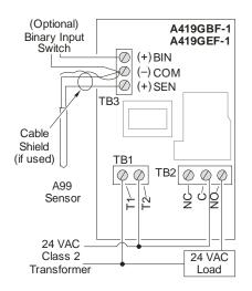
Figure 9: Wiring the 24 VAC A419 Control
