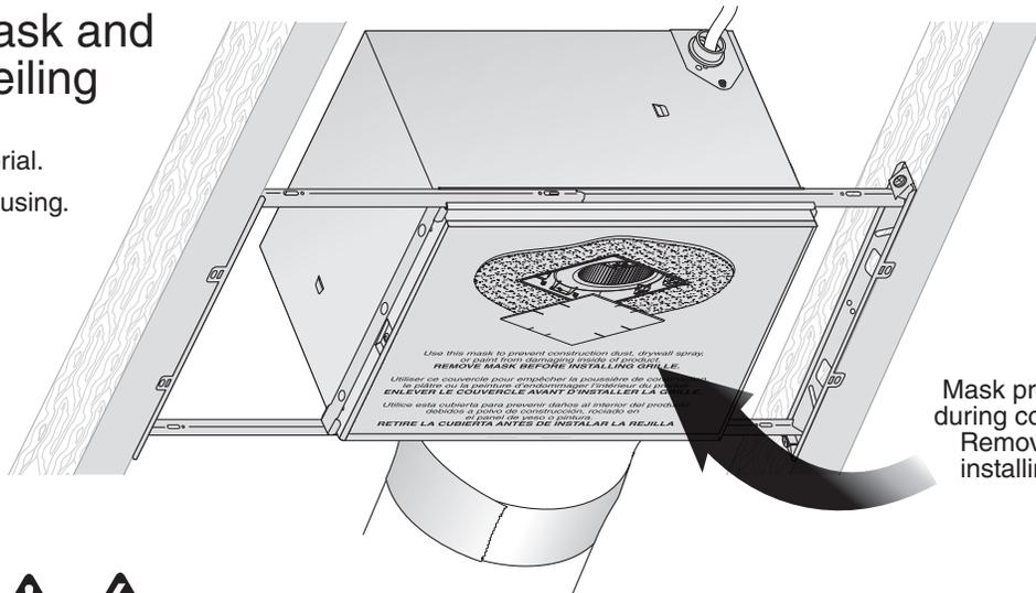
Mask protects unit during construction. Remove before installing Grille.
