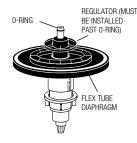
The flush volume of the flex tube diaphragm kit is controlled by the regulator. Regulators are identified by color. Some flex tube diaphragm kits are supplied with multiple regulators. The installer must make sure the proper regulator is used when installing the flex tube diaphragm kit.
