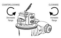
B. Sensor is picking up mirror or highly reflective wall or surface in front of fixture. Install Optima Plus® slightly "off-center" (2 to 5 degrees) to eliminate direct reflection off of mirror or opposite wall or surface.
