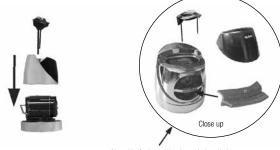
Note. Verify that rubber insert is installed
