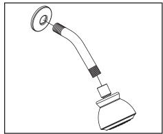
(7) Apply Teflon tape on both thread ends of the (8) For copper pipe, please see the distance shower arm and install shower arm and shower head.
