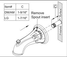
(9) For pipe thread nipple, remove spout insert and apply Teflon tape on the thread end of the nipple, please see the distance charts on the installation instruction pictures for correct installation for each series of tub spout.
