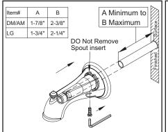
charts on the installation instruction pictures for correct installation for each series of tub spout.
