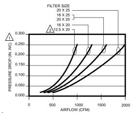
1\text{\frac{1}{1}} WHEN FIRST INSTALLED. PRESSURE DROP INCREASES AS FILTER BECOMES LOADED. REPLACE FILTER WHEN PRESSURE DROP REACHES 0.5 IN. WC. (0.1 kPa).
