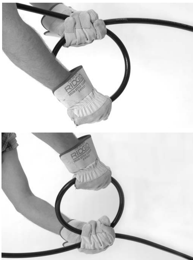
Figure 15 – Rotation du tuyau haute-pression
