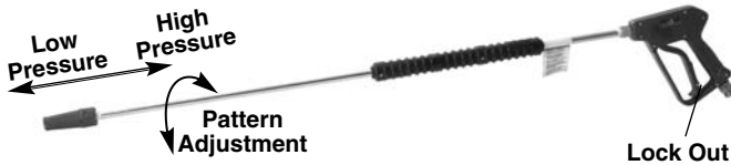
Figure 17 – Wash Wand Nozzle Adjustments
