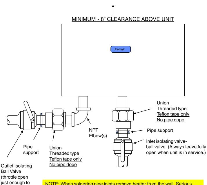
NOTE: When soldering pipe joints remove heater from the wall. Serious damage can occur if any soldering is done while pipes are connected to the heater.
