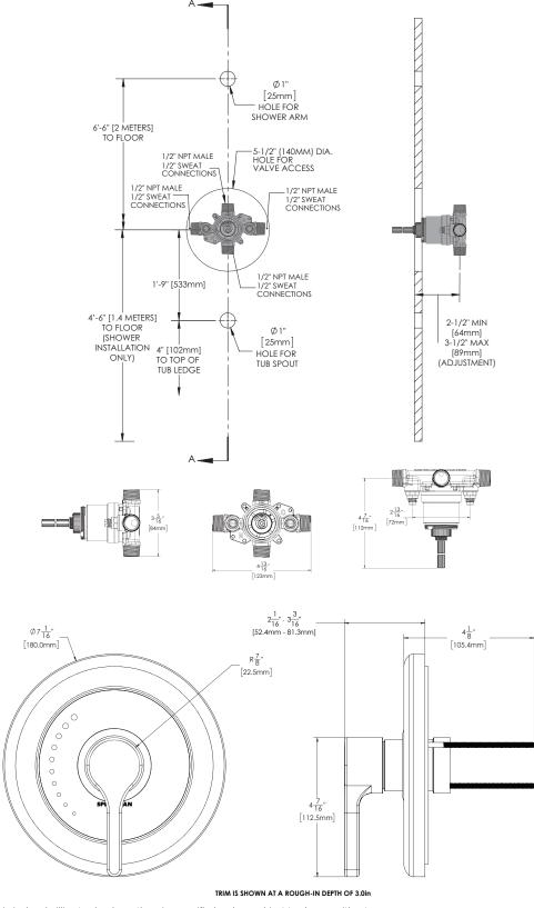
NOTE: 1. All dimensions are in inches (millimeters) unless otherwise specified and are subject to change without notice. 2. Unless otherwise specified, all inlets and outlets are 1/2" female copper sweat. 3. For ADA mounting locations, consult ADAAG, ANSI A117.1, or static regulations
