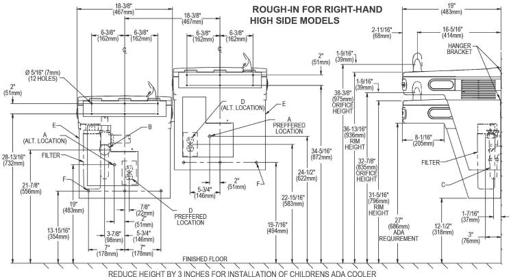
A = Recommended water supply location. Shut off valve (not furnished) to accept 3/8" O.D. unplated copper tube. 3" (76mm) maximum out from wall. B = Recommended location for waste outlet 1-1/2" O.D. drain. Drain stub 2" (51mm) out from wall. C = 1-1/2" Trap not furnished.
