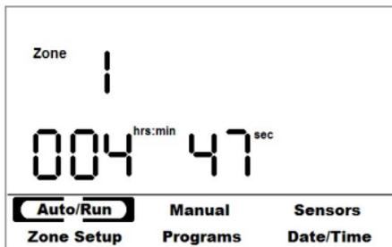
When the controller is watering the zone watering is displayed as well as a count down of the run time.
