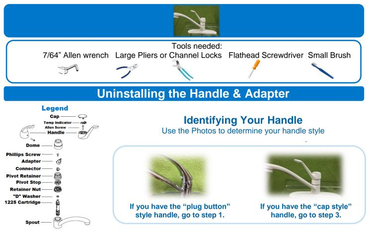
1. Using fingers or a flathead screwdriver, pry off the Moen plug button from the front of the handle. Use a 7/64" Allen wrench to remove the screw. If there are two holes, the screw will be in the larger hole. Then, lift off the handle.
