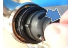
8. Using the grey assembly tool (if available) or a wrench, tighten the cartridge nut until snug. Next turn an additional 90 degrees to fully secure the nut.
