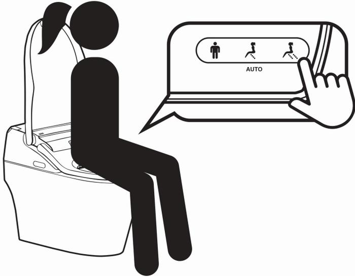
**Note:** To find the suitable level and temperature of the rear and front cleaning combination it is required that the User be seated and using the function. This may require some time to figure out the desired temperature settings. The Water temperature for both the front and the rear cleans is automatically set at 90deg(F) and the Blower default temperature is 180.
