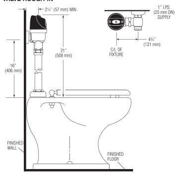
The Model 8113 valve is designed for installations where toilet seat with covers are being used.
