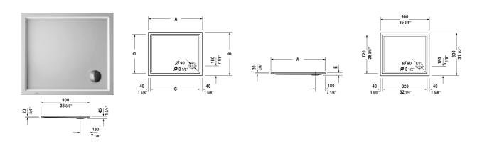
All drawings contain the necessary measurements which are subject to standard tolerances. They are stated in inch & mm and are non-binding. Exact measurements, in particular for customized installation scenarios, can only be taken from the finished ceramic piece.
