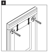
Use adjustment tool to move mirror up and down for leveling.
