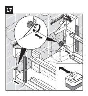
Check the vaniry is leveled and make adjustments using screws.
