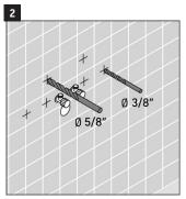
Using a 3/8" and 5/8" drill bit, drill the anchor holes that have been marked.
