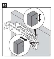
Check the screws which allow adjustment of the unit. the top screw will adjust up and down and the bottom screw will adjust front to back.
