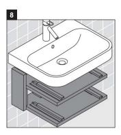
Slide the vanity under the washbasin. Tighten mounting nuts with a wrench until the washbasin is stable.
