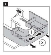
Push and lock in pins, (1) and remove the drawer. (2)
